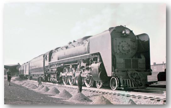
This is the first-ever Niagara, 6000, waiting at the curved part of the Englewood platform to go east. It is a little later than the test era, as the elephant ear-like smoke deflectors are on it, but could well have been among the first revenue trips of the engine. Based on the baggage car, this might be the Fast Mail or it could be the Century with heavy front-end business.
