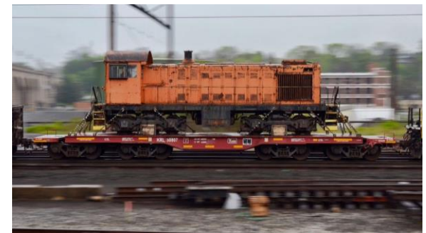
SWITCHER TRANSPORTED ON FLAT CAR
