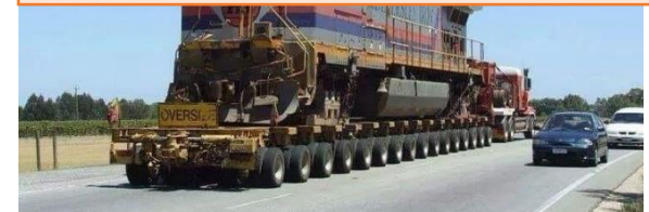
ROAD UNIT TRANSPORTED ON A TRUCK CENTIPEDE FRAME
