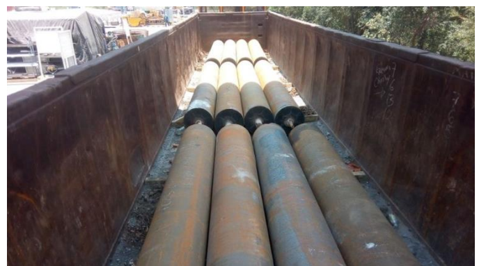
Not every load is visible from the side view as these mill rollers carried by a gon show
