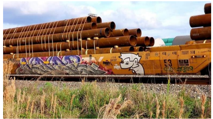
Two well-cars with pipe loads.... Note the offsetting of the tie-down bands and the wood spacers used to secure the loads
