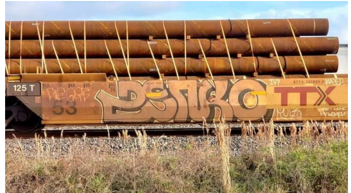
Two well-cars with pipe loads.... Note the offsetting of the tie-down bands and the wood spacers used to secure the loads
