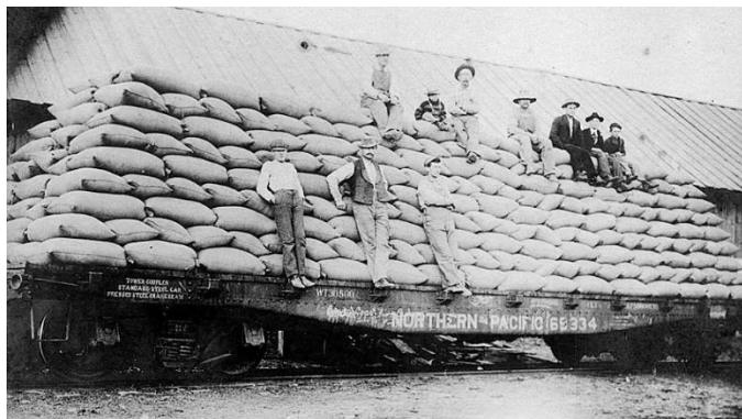
A Vintage photo of a flat car loaded with sacks of wheat circa 1915... note the absence of blocking and tie-downs
