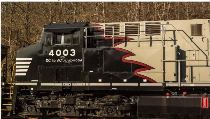
AC44C6M #4003 rebuilt form GE C40-9 Grey with Black mane and Red trim Paint
