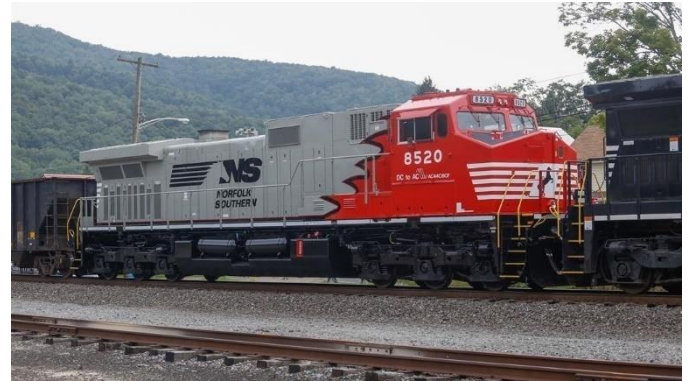
AC44C6CF #8520 rebuilt form GE C44-9W Grey with Red mane and Black trim
