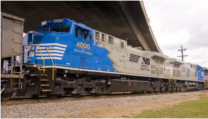
AC44C6M #4000-4001 rebuilt form GE C40-9 Grey with Blue mane and yellow trim Paint
