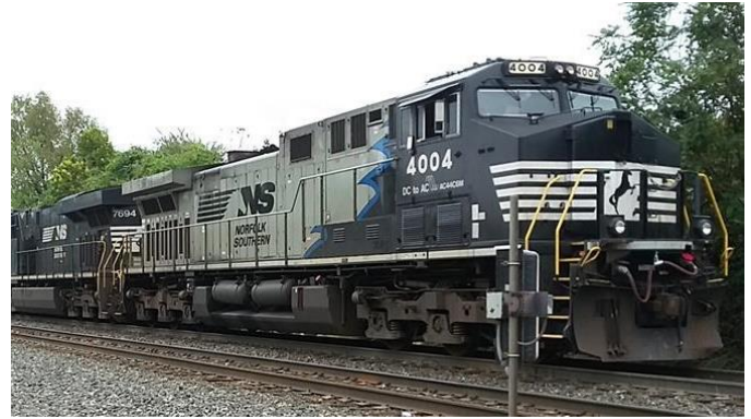
C44C6M #4004 rebuilt form GE C40-9 Grey with Black mane and Blue trim Paint
