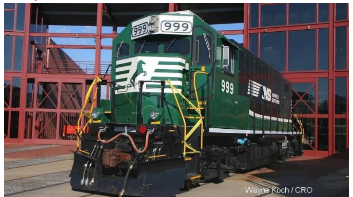
NS # 999 Experimental Battery power Unit
