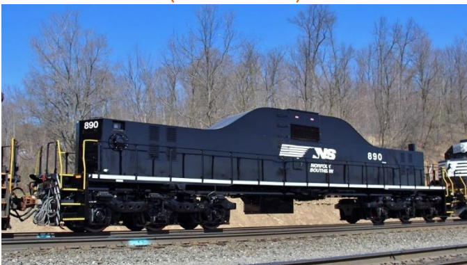
RPU6D #890 Yard Slug in NS Thoroughbred Paint for use with EMD SD33ECO
