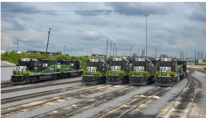
GP33ECO Tier 3 Locomotives rebuilt from SD50 units (#'s 4700-4727)
