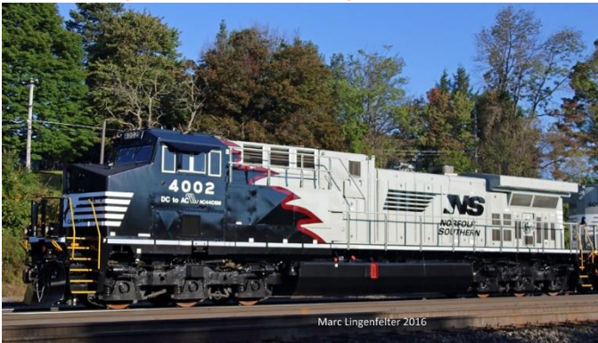
AC44C6M #4002 rebuilt form GE C40-9 Grey with Black mane and Red trim Paint
