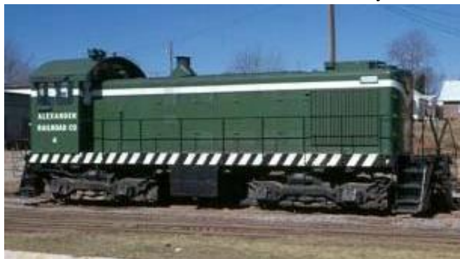
Number Four was an Alco S2 purchased in 1972. Due to her weight, she was sold less than a year later.
