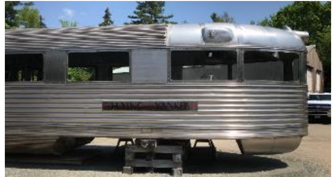
Observation Car from the Flying Yankee Streamliner sans windows and trucks is undergoing restoration
