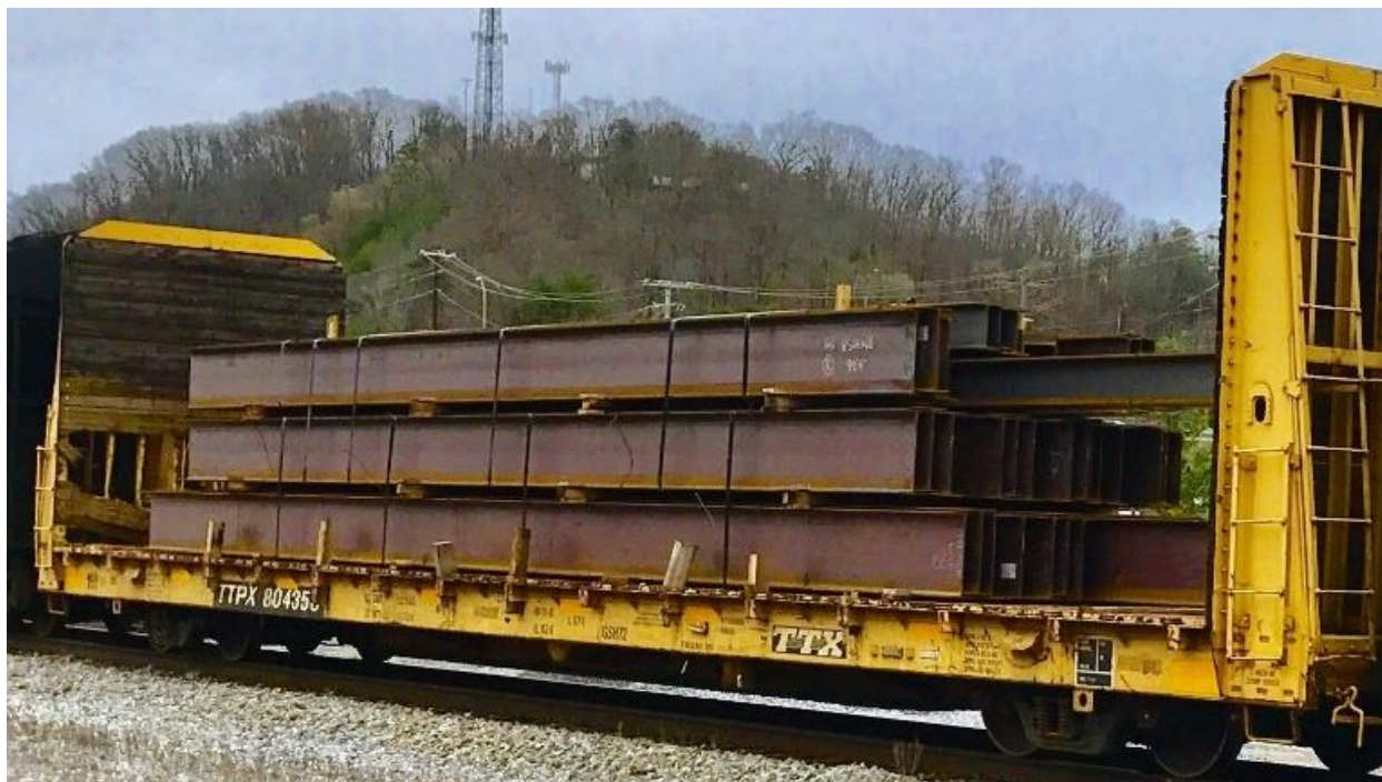
THE TTPX 804358, A BULKHEAD FLAT CAR CAUGHT THE ATTENTION OF PAUL HAYNES AS IT PASSED THROUGH THE TRI-CITIES. ITS BATTERED FLOORING AND BULKHEAD ENDS ALONE WOULD HAVE MADE IT A CANDIDATE FOR MODELING. HOWEVER, ITS LOAD OF STRUCTURAL STEEL "I" BEAMS MADE IT ESPECIALLY WORTHY OF MODELING IT IN HO SCALE.
