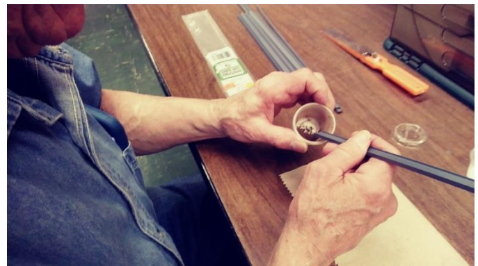
In the photo above Paul is applying the iron oxide to ends of the beams
