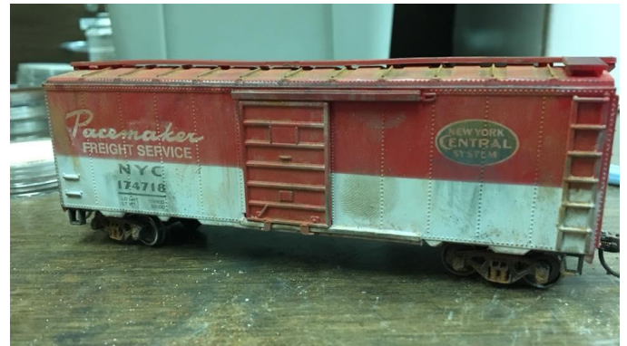
Here's the finished car, Logan's first attempt... it took about 30-45 minutes to complete with 25-30 minutes wrapped up in drying time for the Dul-Cote applications
