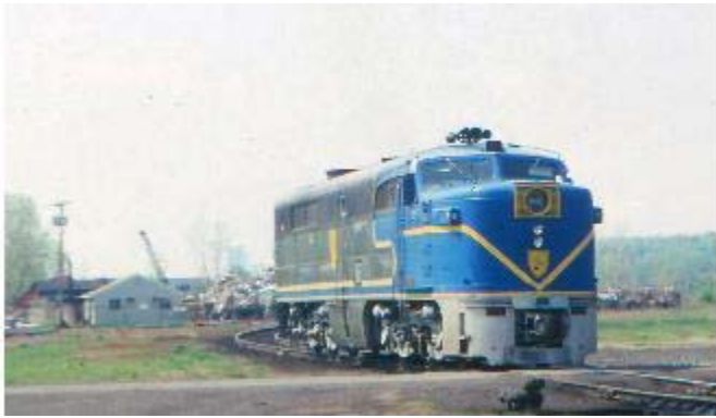
Alco #16 coming toward the depot from the engine house. The engine was re-motored from its original powerplant to a later Alco 251V12 in 1974-75, just before this trip.
