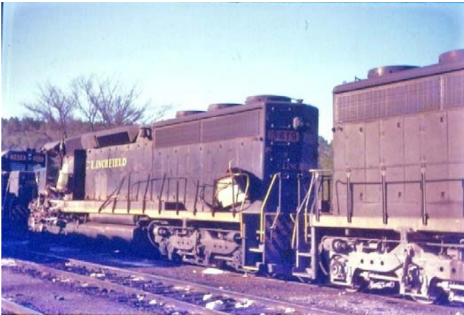
3619 is being towed back by a sister SD. It will be several months before 3619 receives a new cab and rebuild and is returned to service.
