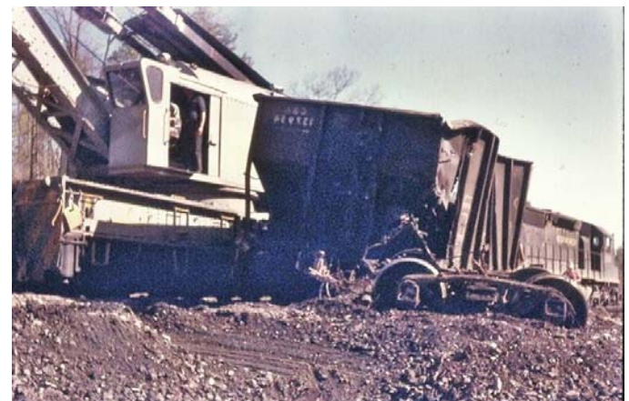
Rolling stock took heavy damage as evidenced by the bent and twisted hopper cars pushed aside and shorn of their trucks.
