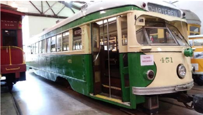
Looks like a bus, but is an excellent example of a PCC car.
