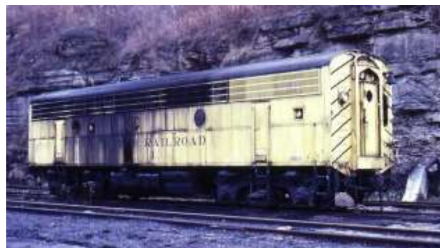
A view of the fireman's side of the cab of Haysi #1- note the scorch marks from the engine fires #1 was prone to late in life - Photo from Clinchfieldcountry.com.
