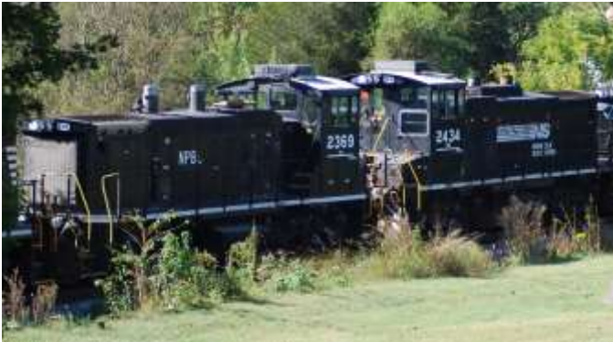
#2434 & 2339 MP15DC built for SR received in 1982 1500 hp
