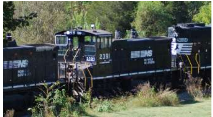
#2391 MP15DC built for SR received in 1982 1500 hp
