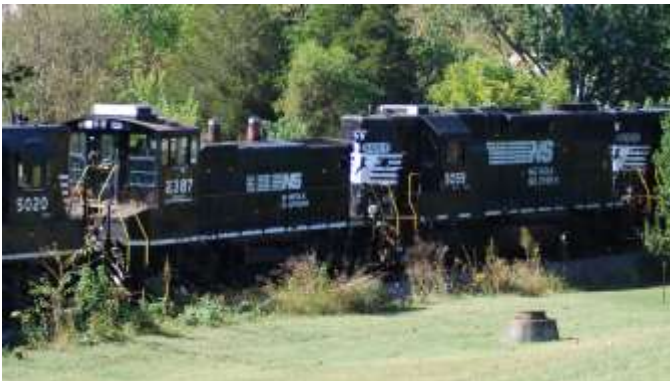
#5020 GP38-2 build for SR received in 1982 2000 hp #2387 MP15DC built for SR received in 1982 1500 hp
