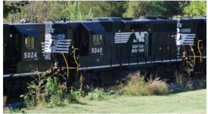
#5040 GP38-2 build for SR received in 1982 2000 hp
