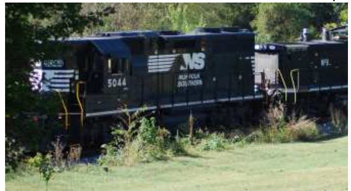
#5044 GP38-2 build for SR received in 1982 2000 hp
