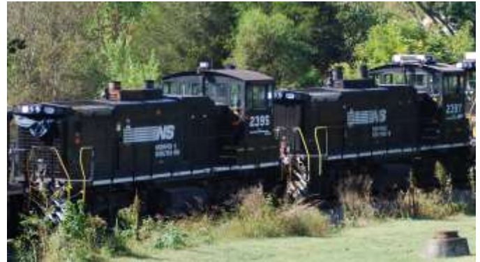
#2397 & 2395MP15DC built for SR received in 1982 1500 hp
