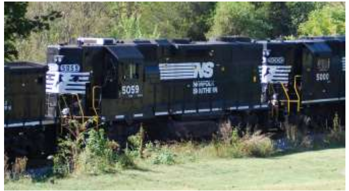
#5059 GP38-2 build for SR received in 1982 2000 hp
