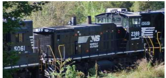
#2389 MP15DC built for SR received in 1982 1500 hp
