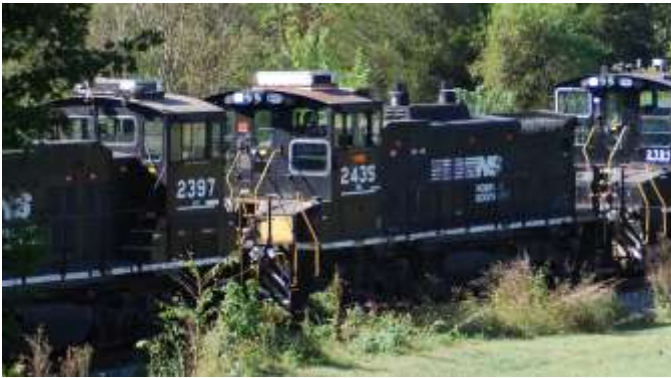
#2435 MP15DC built for SR received in 1982 1500 hp
