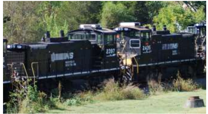
#2435 & #2397 MP15DC built for SR received in 1982 1500 hp
