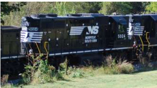
#5024 GP38-2 build for SR received in 1982 2000 hp
