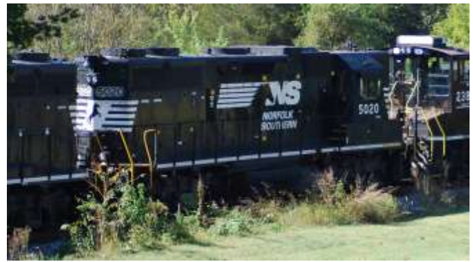
#5020 GP38-2 build for SR received in 1982 2000 hp
