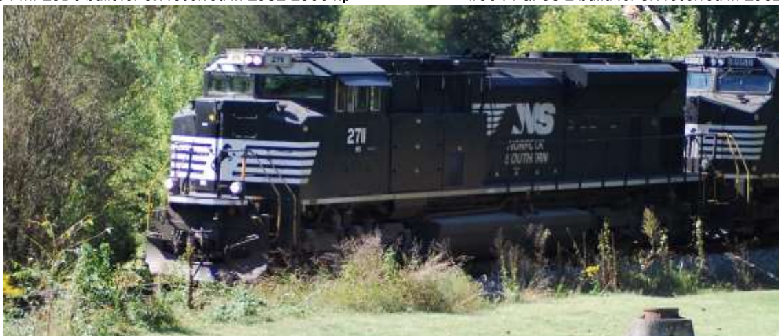
HEADING EASTBOUND NS #2711, A EMD GP35 FIRST BUILT FOR THE SOUTHERN IN 1965 RATES 2200 hp
