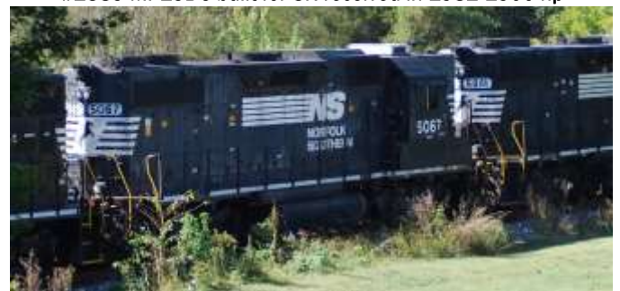
#5067 GP38-2 build for SR received in 1982 2000 hp
