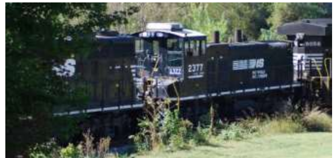
#2377 MP15DC built for SR received in 1982 1500 hp
