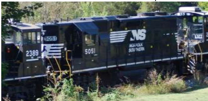
#5051 GP38-2 build for SR received in 1982 2000 hp
