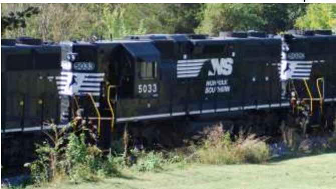
#5033 GP38-2 build for SR received in 1982 2000 hp
