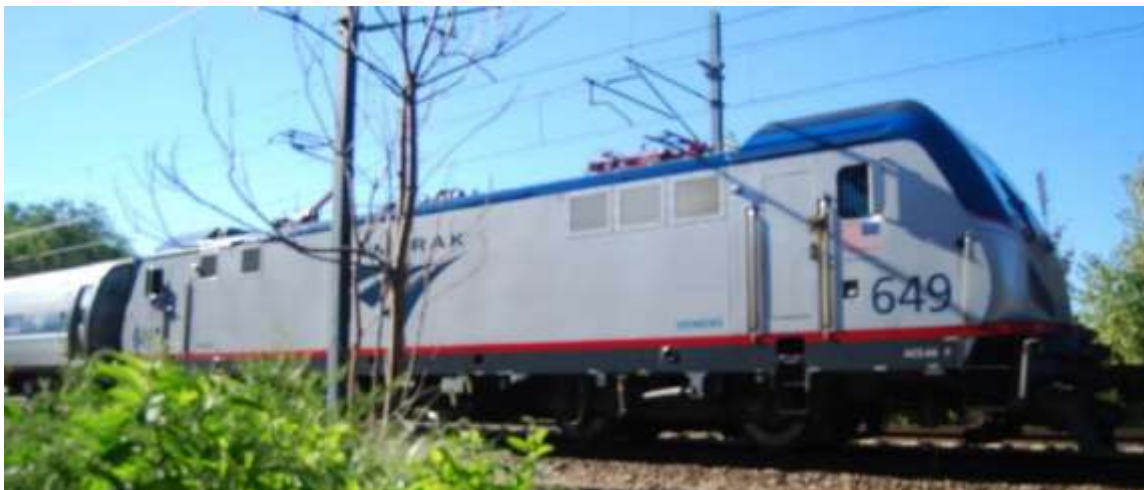
Amtrak #649, a Siemens ACS-64 electric locomotive powers its train southbound in the Northeast Corridor just East of Mystic Connecticut. In about 1 mile it will slow from 70 mph to a stop at the station in Mystic using the former New Haven mainline between Boston and New York City.
