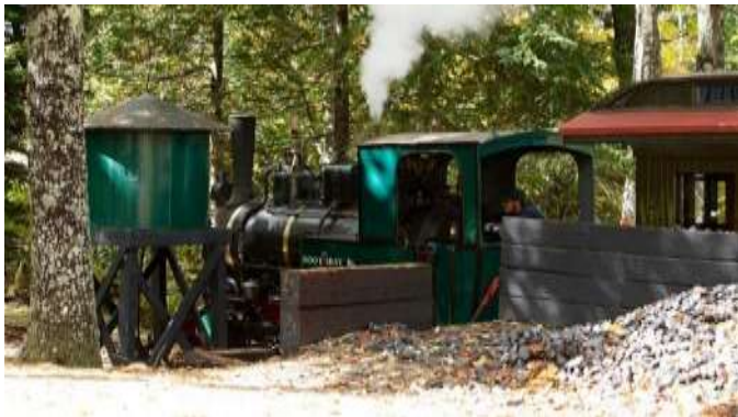
The Coal Bin, the engineer will stop from time to time to replenish the engines coal supply. The Water Tower provides water for the locomotive's storage tank. During operation water is forced into the boiler to provide for steam generation Photo Courtesy of railroadvillage.org.
