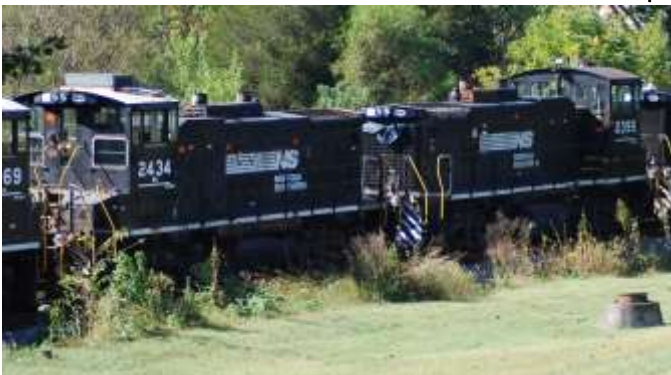
#2395 & 2434 MP15DC built for SR received in 1982 1500 hp
