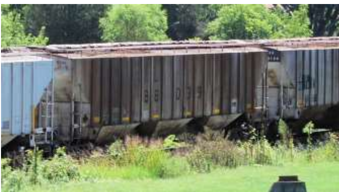
Weathering on Southern RY #88093 (LO Covered Hopper) has all but obscured the car's road name lettering.
