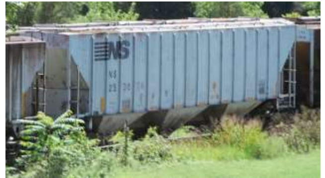
Norfolk Southern #253078 shows only slight weathering save for the obscured reporting marks on the top end panel... yellow safety reflector stripes have been applied
