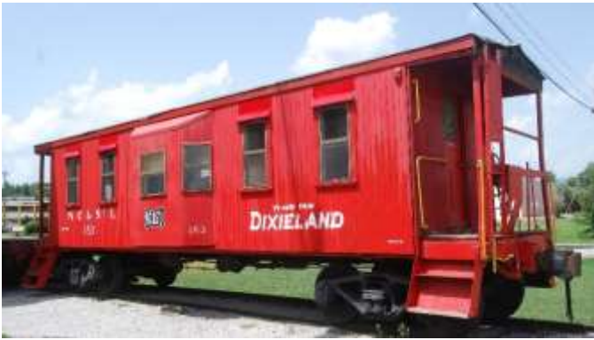
NC&StL Caboose #153 is a unique piece of rolling stock. It has a steel frame, wood sheath sides, and metal bay windows added
