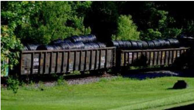
KCSM (Kansas City Southern de Mexico) #61314 and GRW (Gary Railway Co.) #87699 carry open loads of coiled steel... the coils are secured only by their weight
