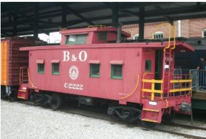
B&O caboose C2222 is an example of a steel frames wood-sheathed caboose operated by the B&O
