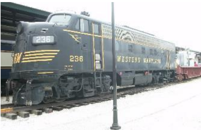
Western Maryland No. 236 is an example of a first generation 1500 hp F7.
