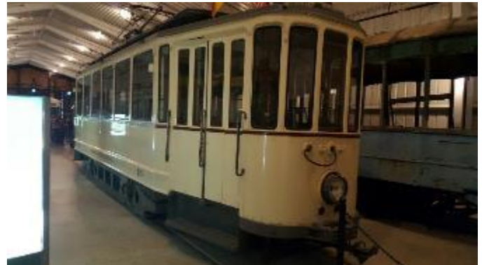
Rheinische Bahngesellschaft 955, made by Gebruder Schondorff AG in 1928, Dusseldorf, Germany. It features a single truck, double end, City-suburban tram with two motors and trailer connections
