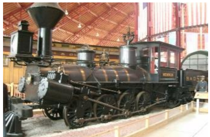
The museum host displays of some of the earliest examples of locomotive and rolling stock. "Memnon" #57, an 0-8-0 built in 1848 by Newcastle Mfg., one of the oldest surviving freight locomotives on display.
