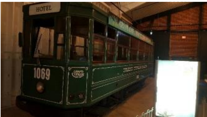
Here is an example of a wood street car. It's a Société des Transports Intercommunaux de Bruxelles (STIB) 1069, built by Les Ateliers Métallurgiques de Nivelles, 1907 in Brussels. Its principal features are: Single truck-single end design.
