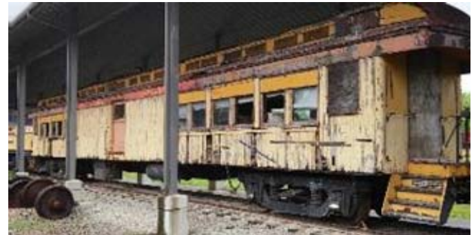
Of historical significance is the Louisville and Nashville Combine Car Number 665. It was one of only two "two wood side steel" train cars ever made (the second car is located at the Bowling Green RailPark and is in a much better state of preservation). It was designed for the times of the Jim Crow laws; whichever end was the front during the trip would hold white passengers, while the rear held black passengers. It was given to the Kentucky Railway Museum by the Louisville and Nashville Railroad in 1958. [16] During the Civil War Centennial observances of the 1960s this car was pulled by the famous Civil War-era steam locomotive The General, touring various parts of the Eastern U.S. rail network.
