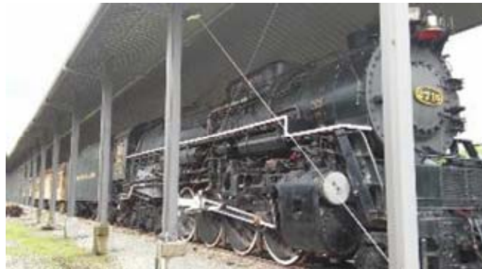
C&O 2716, a 2-8-4 Kanawa class locomotive built by Alco for the Chesapeake & Ohio Railroad in 1943 is one of those exhibits. The unit is currently non-operable.
