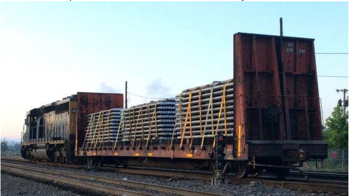
The CSX switcher at Kingsport TN pulls Illinois Central Gulf bulkhead flat car (ICG 978920) with a load of aluminum rods Photo by Paul Haynes
