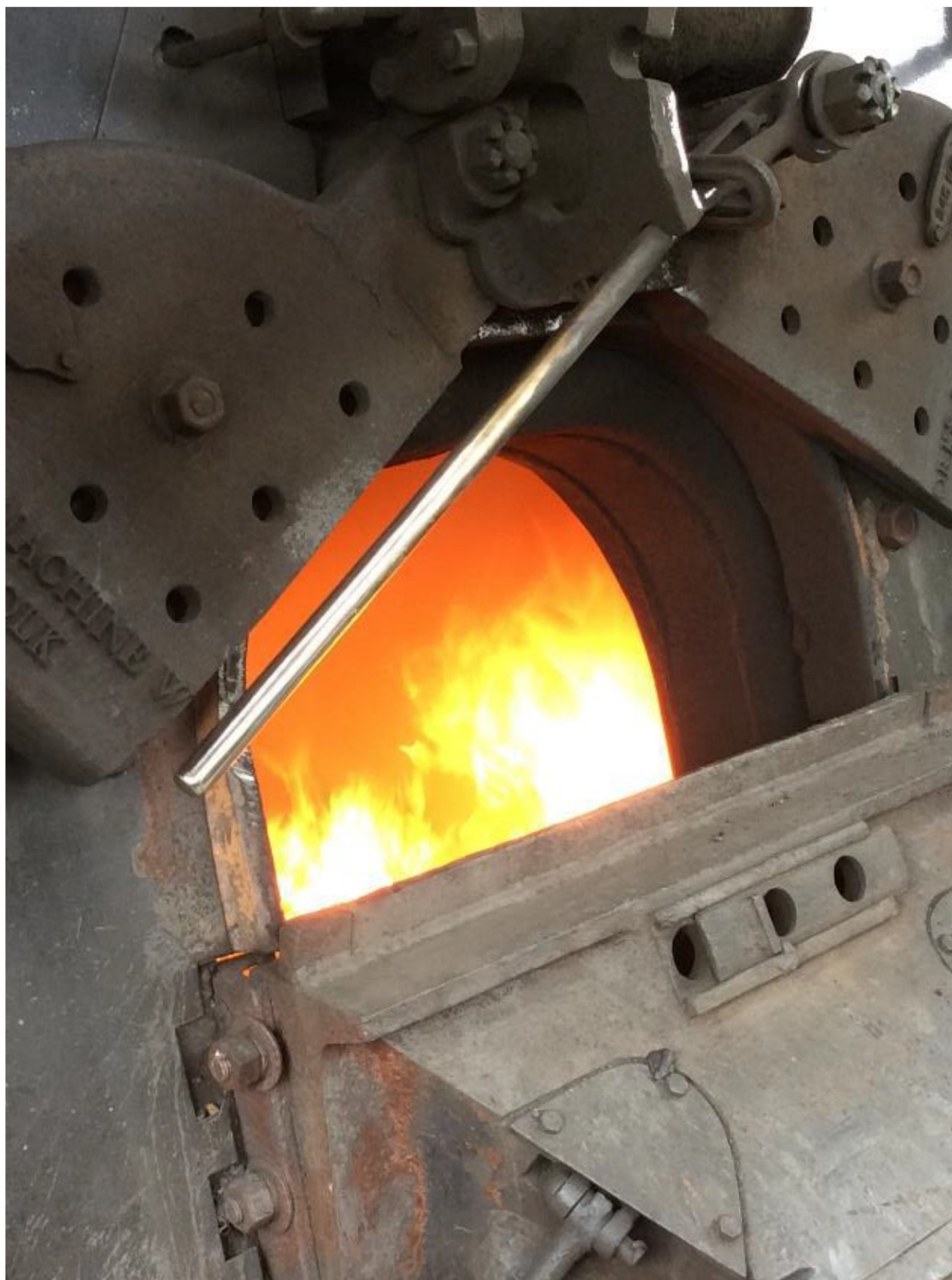
A fiery "Hell on Wheels" – a view of N&W 611's firebox while under steam
