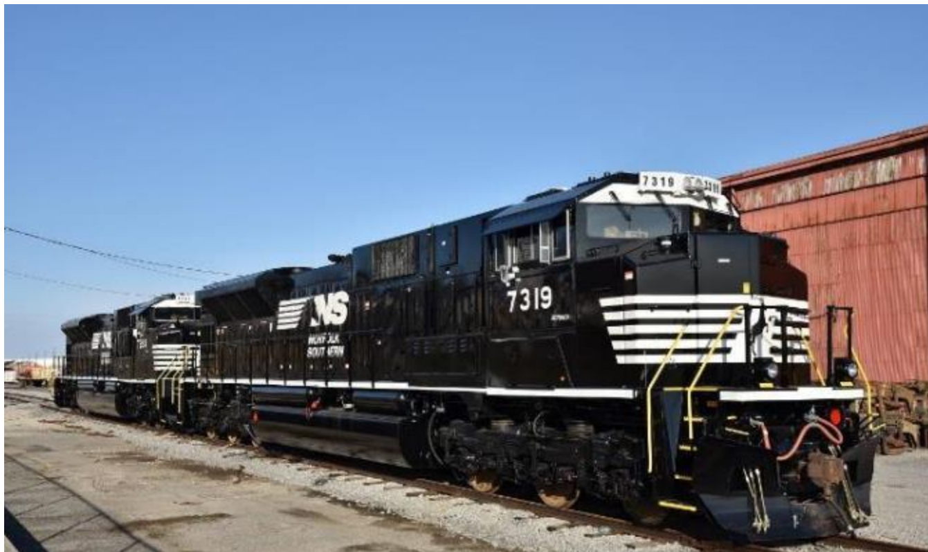
Norfolk Southern SD70ACU No. 7319 is ready, but not released for service, at the railroad's shops in Altoona, Pa. The railroad has already completed two refits from SD90MACs. Photo by L.R. Myers of AltoonaWorks.info
