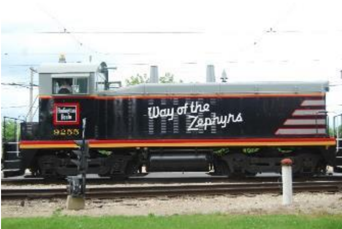
Built in 1950, CB&Q's #9255 shows the evolution of the yard switcher as a SW-7 wearing Burlington's attractive black-grey-red-and- orange paint.
