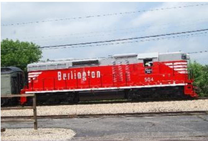
Chicago Burlington and Quincy #504 is an EMD SD-24 built in 1959 and restored in the CB&Q red-grey-and-white paint scheme
