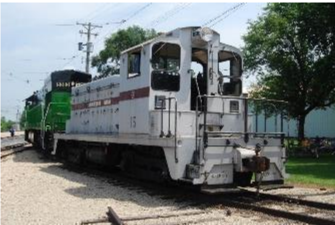
Commonwealth Edison's #15, an EMD SW1, is a fine example of a first generation switcher
