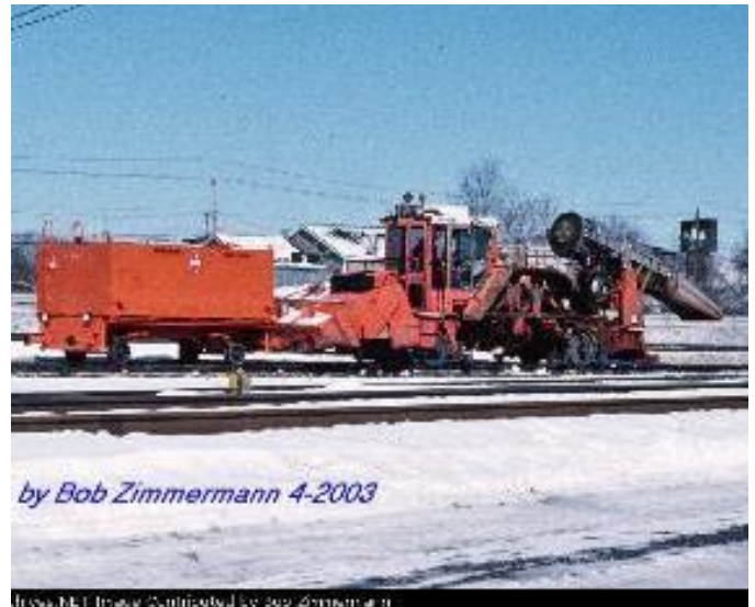
NS BR920058X (Snow Plow) snow melter working NS Gang Mills yard early 2003; no actual markings for NS. Smelled like jet fuel.
