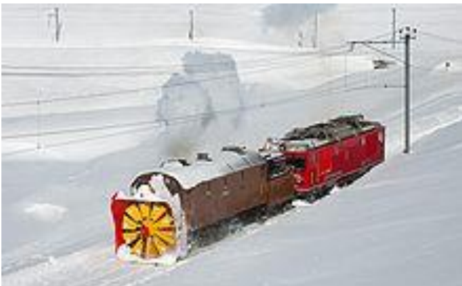
Operational rotary snowplow Xrotd 9213 of Rhaetian Railway
