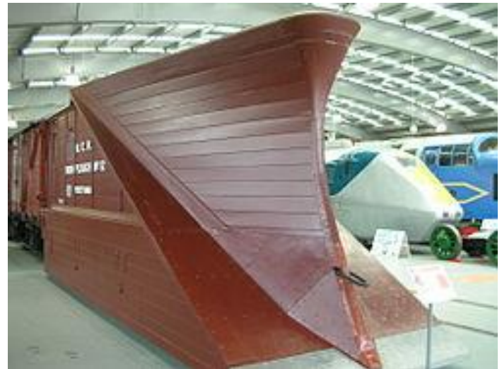
An example of a railroad wedge plow
