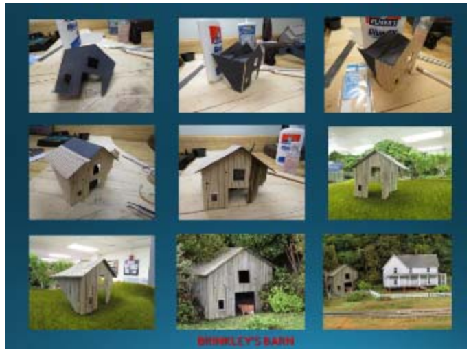
This collage of photos quickly steps you through the major steps of construction of the Brinkley barn. From top left to lower right: the cardboard base of the barn painted black to make the cardboard less absorbent to the white glue that will be used to fix the wooden strips on the base. The barn is not a complete square/rectangular structure, but is designed to fit into the scenery at a 45 degree angle and on a slanted surface. This can be seen in photos 2 and 3. Scale Lumber strips are being applied to the cardboard base with Elmer's white glue. Campbell paper shingles are applied to the roof using white glue. The wood exterior is stained with a series of acrylic paint washes and then overwashed with a diluted India ink wash to create an aged appearance. The barn in place and scenery placed around it to blend it into the small space it will occupy on the
