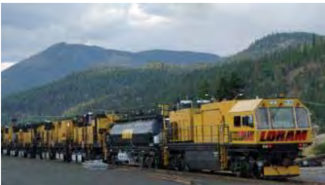
A Loram Rail Grinder in transit
