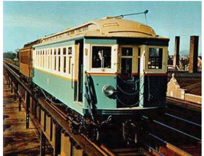
Car 1812 breezes along at Homan on the Lake Street Line in mid-1950. Car 1812 began as Northwestern trailer 273 (later 1273) in 1907. In 1950, it and six identical cars were converted to motor cars (1809-1815) at the West Shops. Car 1812 was livered with the Mercury Green, Croyden Cream and Swamp Holly Orange, standard on PCC streetcars since 1946. No other wood cars were so painted, but the scheme was adopted for the 6000-series in 1950.
