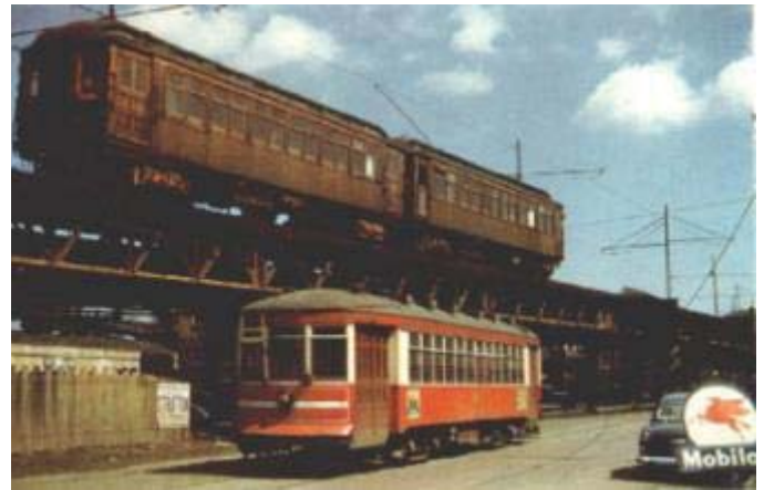
In 1949, a train of a 1906 Jewett-built and a 1903 St. Louis-built "L" car, then still operating from overhead trolley wire, overtakes a 1923 Brill-built streetcar on the Lake Street Line.
