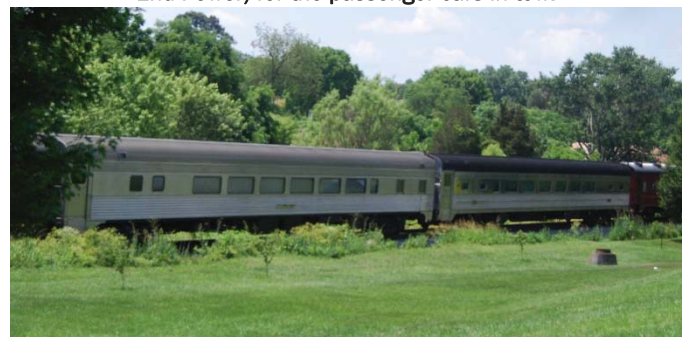
The tool car is trailed by a generator car to provide HEP (Head-End-Power) for the passenger cars in tow.
