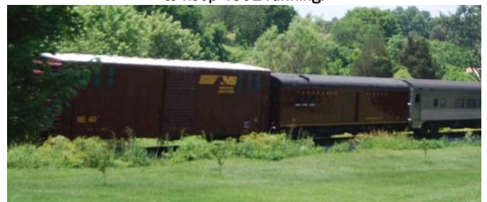
The tool car is trailed by a generator car to provide HEP (Head-End-Power) for the passenger cars in tow.
