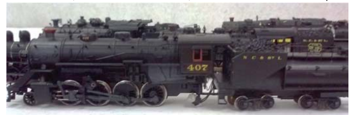
Part of Tom Knowles NC&StL Locomotive collection – foreground is 2-8-0 #407 with lightly modified Vanderbilt tender and boiler with a typical NC&StL capped stack.
