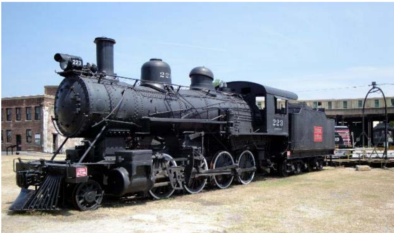
Central of Georgia Railway locomotive no. 223 in front of the roundhouse at the Georgia State Railroad Museum (Roundhouse Railroad Museum), Savannah, Georgia, USA. The roundhouse is part of the CG Savannah Shops Complex, built in 1853. The locomotive is a Baldwin C-3 class 2-8-0, built 1907, retired from service in 1952.
