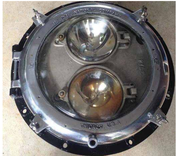
A preview of things to come – 611 will received a new dual beam headlamp assembly – the housing appears newly chromed ready for instillation.
