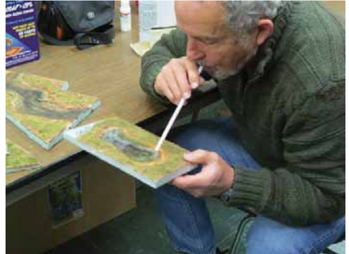
Bubbles are removed by blowing through a straw directed towards the water and held just above it. The carbon dioxide in your breath removes the tiny bubbles.
