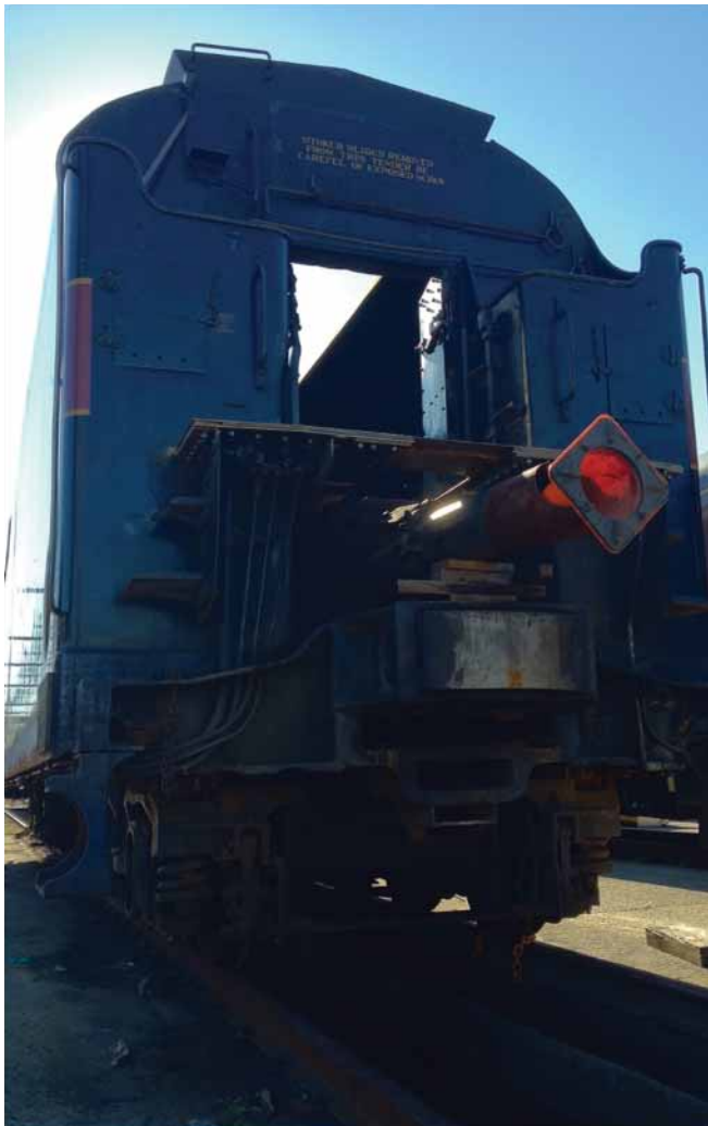
The auger pipe for the automatic stoker is visible in this shot (see the red safety cone)
