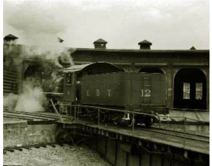
Coming from a brick roundhouse stall with 'modern' rollup doors (1920s) is Mike #12, the first such wheel configuration the line bought and delivered in 1911; they ended up with seven total. New FRA rules on flue time have made getting any of the locomotives running again a very expensive task; #15 is reportedly the 'sole survivor' in that regard.
