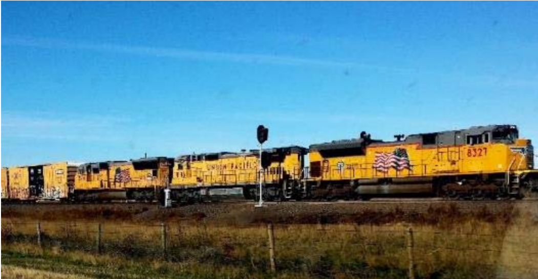
An eastbound Union Pacific manifest train passes along I-80 in Wyoming. The train is led by an EMD SD70ACe with an older Dash-8 second in line. An SD70M with flared radiators is the third locomotive in the consist
