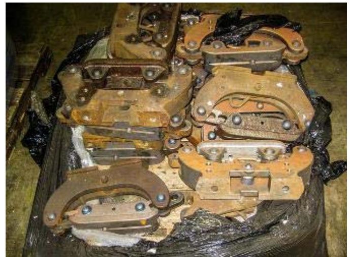
Third Rail Shoes Ready for installation
