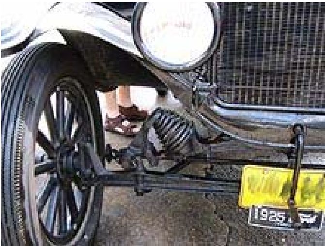
The suspension components of a Ford Model T. The coil-spring device is an aftermarket accessory, the "Hassler shock absorber".
