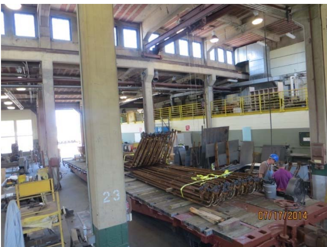
Superheater units for 611
