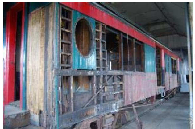
EAST TENNESSEE & WESTERN NORTH CAROLINA COMBINE No 15 UNDERGOING RESTORATION
