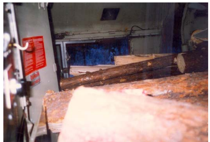
Anywhere there was glass, the pulp logs loaded cross wise on the truck, penetrated into the cab including through the number boards
