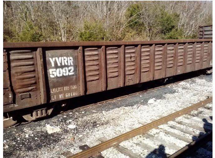
An example of a mill gondola in scrap metal service
