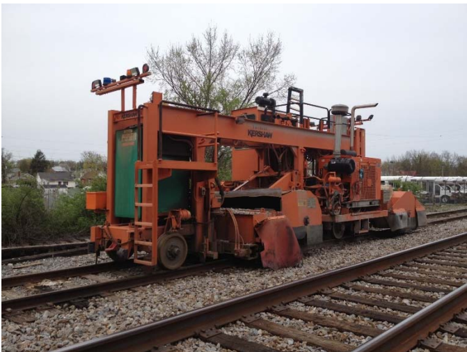
TAMPERS - Maintenance-of-Way (MOW) machines capable of raising, aligning and tamping, and resetting tie and rail assemblies, tampers are one of the most widely used MOW machines.
