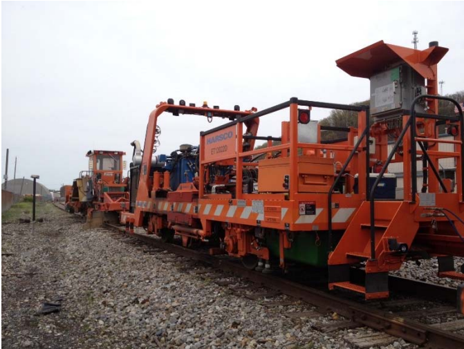
TAMPERS - Maintenance-of-Way (MOW) machines capable of raising, aligning and tamping, and resetting tie and rail assemblies, tampers are one of the most widely used MOW machines.
