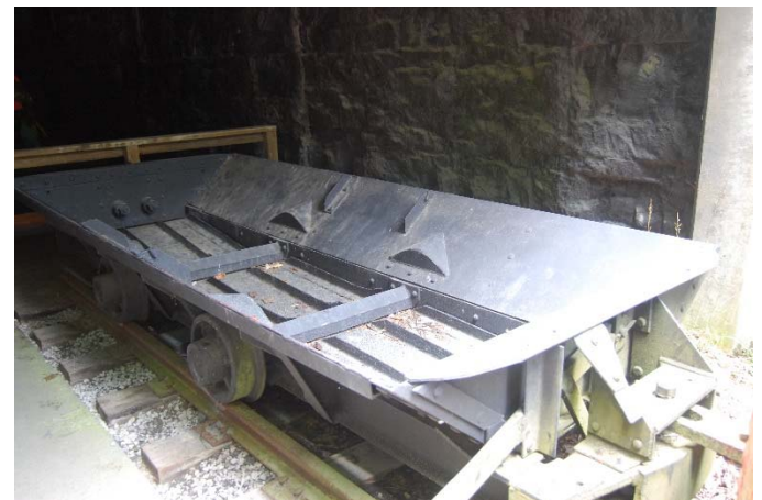
Just inside the mine opening and a short distance away are two ore hoppers. Like the rest of the equipment, they are low squat cars designed to work in the low clearances of the mine itself. The height of the shafts and passageways were dictated by the height of the coal seam. In Blue Heron's case the height was rarely more than 3-4 feet.
