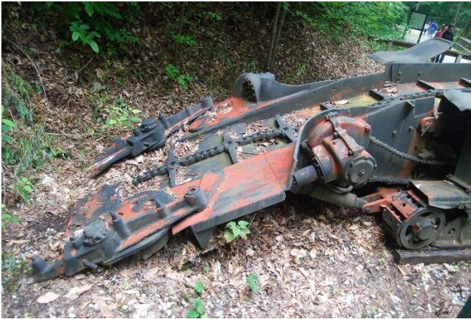
The loader would be moved near the seamface where mechanical arms would scoop the coal broken from the face onto the conveyor belt. Temporary track would be run the the seam face and a hopper positioned to receive its load from the conveyor belt.
