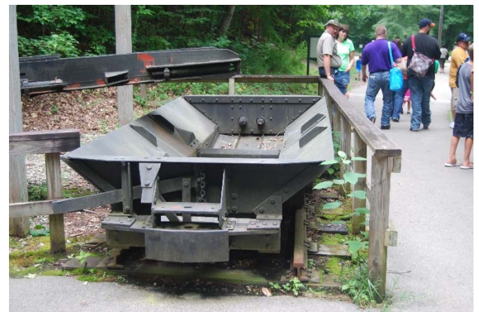
The display also includes a loader with coal hopper positioned beneath the conveyor belt. In the photo below you can see the armatures and poles used to support the wire to power the electric mules.
