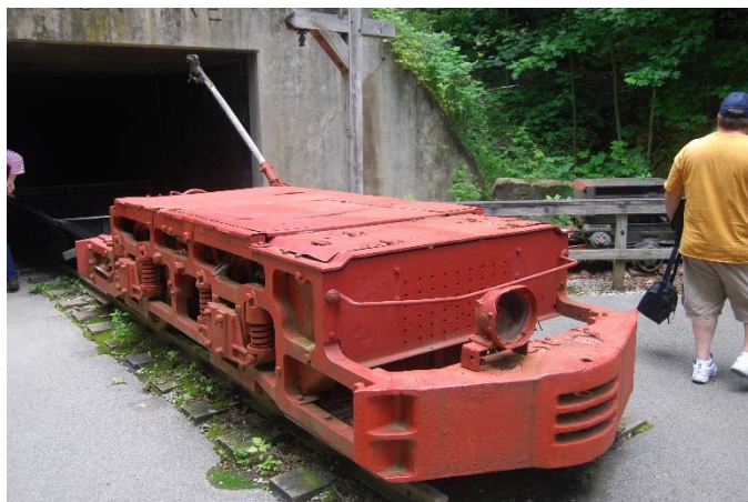
Just outside of the mine entrance is an electric "mule", a powered mine car used to move the ore hoppers to and from
