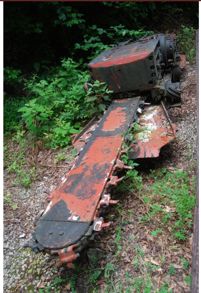
The tool shown above is a seam shear used to undercut the seam face which in turn allowed the miners to drop the coal in the seam above the cut to the mine floor. Chunks could then be broken into manageable pieces and fed to the loader. Remember all this was done at Blue Heron in a passageway 4 foot high from a kneeling position!
