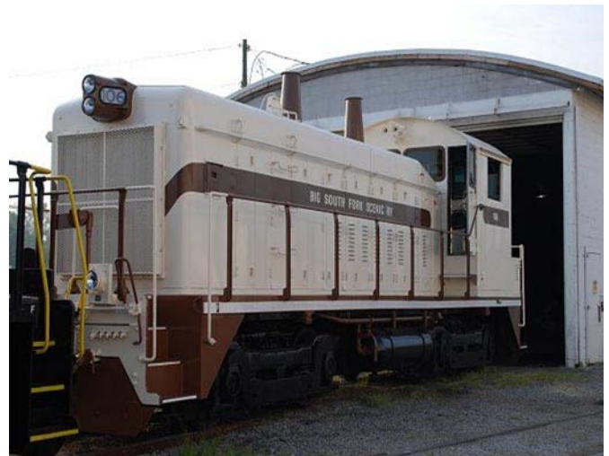
Big South Fork Scenic Railway #106 1951, EMD SW-9, 12 CYL 567B engine and later rebuilt with 12 CYL 567BC, 1200 hp. Ex-Seaboard Coast Lines #183, ex-Laurinburg & Southern RR #138, acquired by Gulf and Ohio in 1997. In Service.
