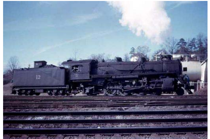
Kentucky & Tennessee Railway #12 photographer unknown 1911, 2-8-2, built by Baldwin, C/N 37085. 27 x 30" cylinders, driver diameter 63". Ex-Sou. Rwy 4501, to Paul H. Merriman/TN Valley Rwy. Museum 1964
