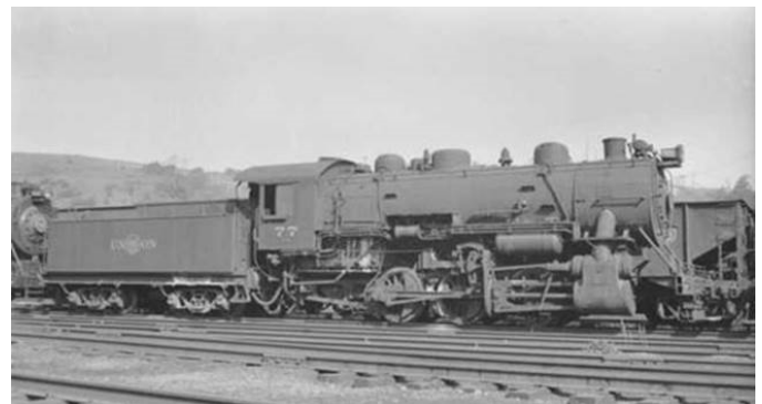
Manufactured by American Locomotive Company, Schenectady, NY 1944 c/n 71323 Wheel Configuration 0-6-0 Weight - 90 tons on drivers Cylinders 22x28" Drivers 51"
