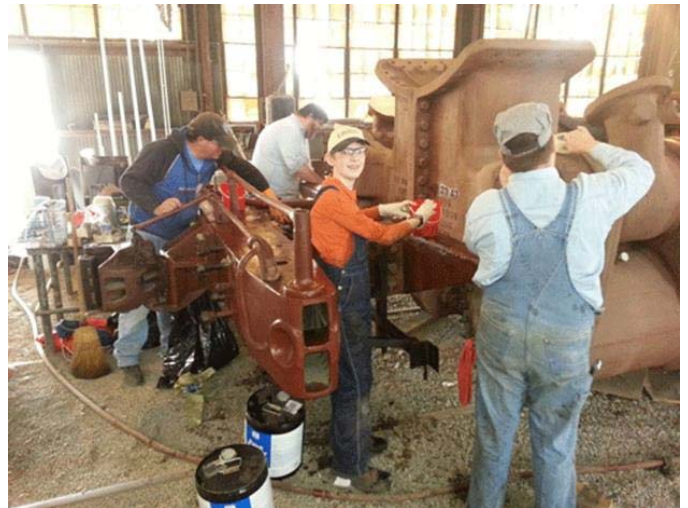
Thomas Bookout and James Hamilton masking rods in preparation for painting of the locomotive frame 4/14/13
