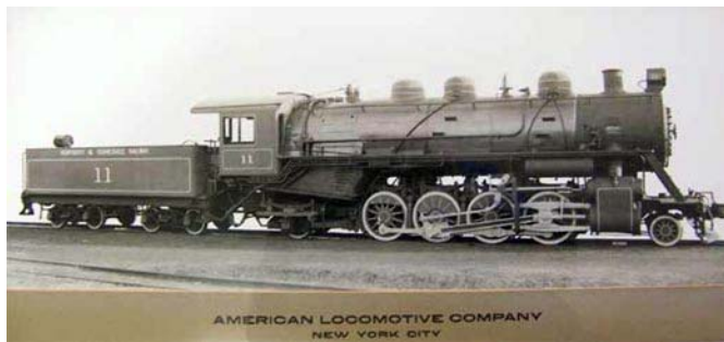
Kentucky & Tennessee Railway #11 builder's photo in K & T Railway Office 1922, 2-8-2, built by Schenectady (ALCo), C/N 63271. 25 x 30" cylinders, driver diameter 56". Purchased new. To Aberdeen Proving Grounds, 1963. Accidentally destroyed by artillery on gunnery range.
