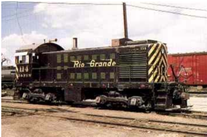
Here's a picture of D&RGW #114 from "Classic Locomotives, the Series". This is how ALCO 102 would have appeared when purchased used by the K & T Railway in 1963. After purchase by the K&T, the exhaust stack was cut down due to the close-clearance tunnel on the K&T.
