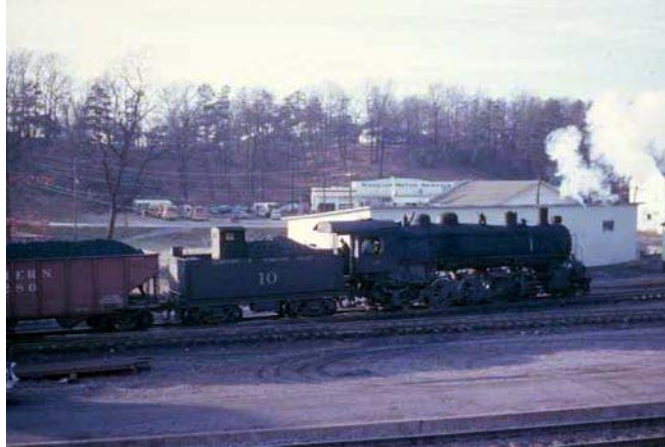
Kentucky & Tennessee Railway #10 photographer unknown 1920, 2-8-2, built by Baldwin, C/N 53182. 24 x 30" cylinders, driver diameter 56". Purchased new. To TN Valley Rwy. Museum 1964
