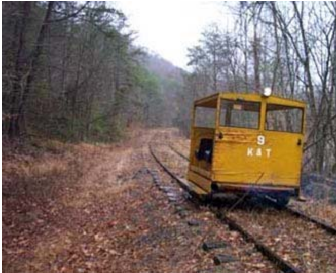
Motorcar 9 is a 1956 Fairmont A3-D that was purchased new by the K & T and was active on the railroad during the steam locomotive era and was primarily used as the Superintendent's inspection car. It is stored in the motorcar barn and is still used occasionally. It is powered by a 4 cylinder Waukesha industrial engine.
