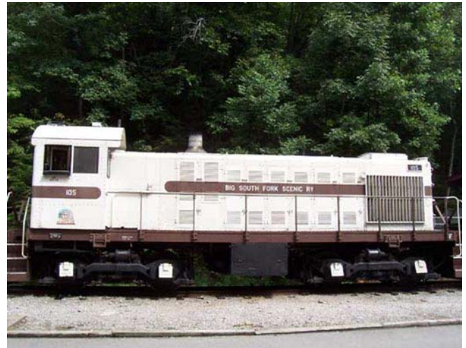
Big South Fork Scenic Railway #105 1942, BB, C/N 70651, built by ALCo, 900 hp . Ex-Port Huron & Detroit RR #60, ex-Genesee & Wyoming. Shop for maintenance.
