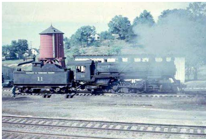
Kentucky & Tennessee Railway #11 builder's photo in K & T Railway Office 1922, 2-8-2, built by Schenectady (ALCo), C/N 63271. 25 x 30" cylinders, driver diameter 56". Purchased new. To Aberdeen Proving Grounds, 1963. Accidentally destroyed by artillery on gunnery range.
