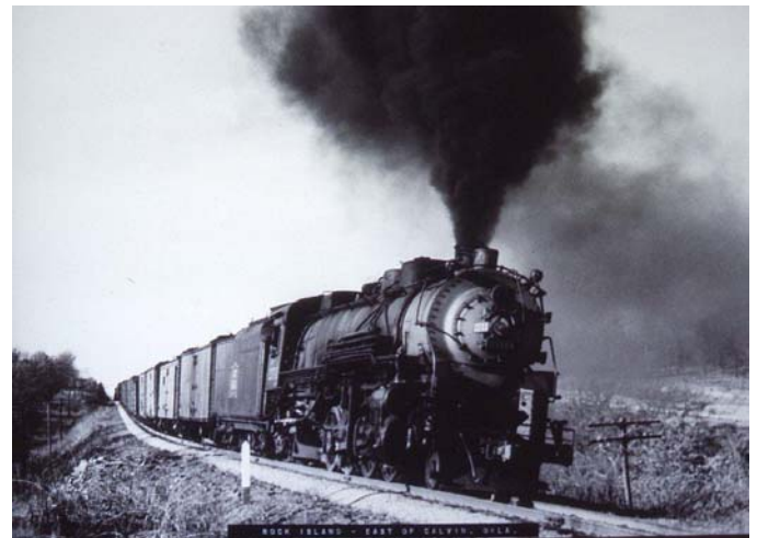
Eastbound Mikado 2711 (2-8-2) at from Hilltop, Okla., at the top of the Shawnee Hills between Calvin and Stuart with 47 cars on Dec 13, 1948
