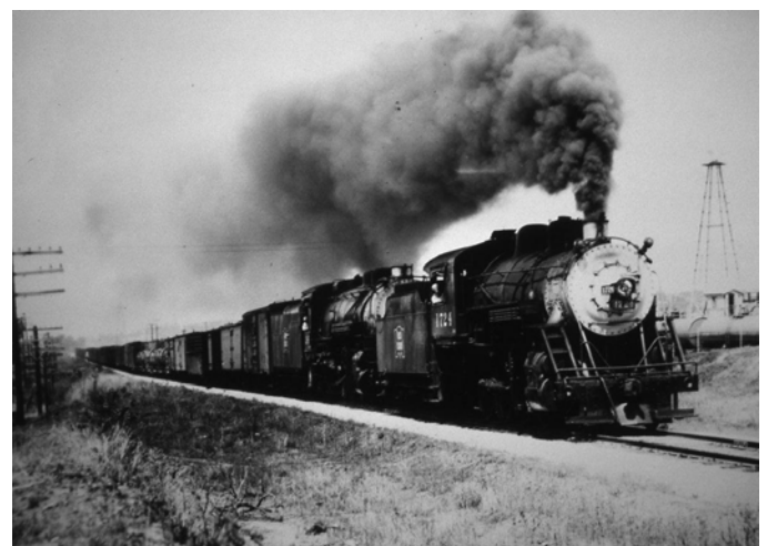
Eastbound Consolidation Double Header #'s 1724 (2-8-0 Consolidation) and 2665 (Mikado 2-8-2) lead an eastbound freight through Seminole, Ok., oilfield on the Choctaw line with 75 cars at 30 mph on Sep 2, 1946
