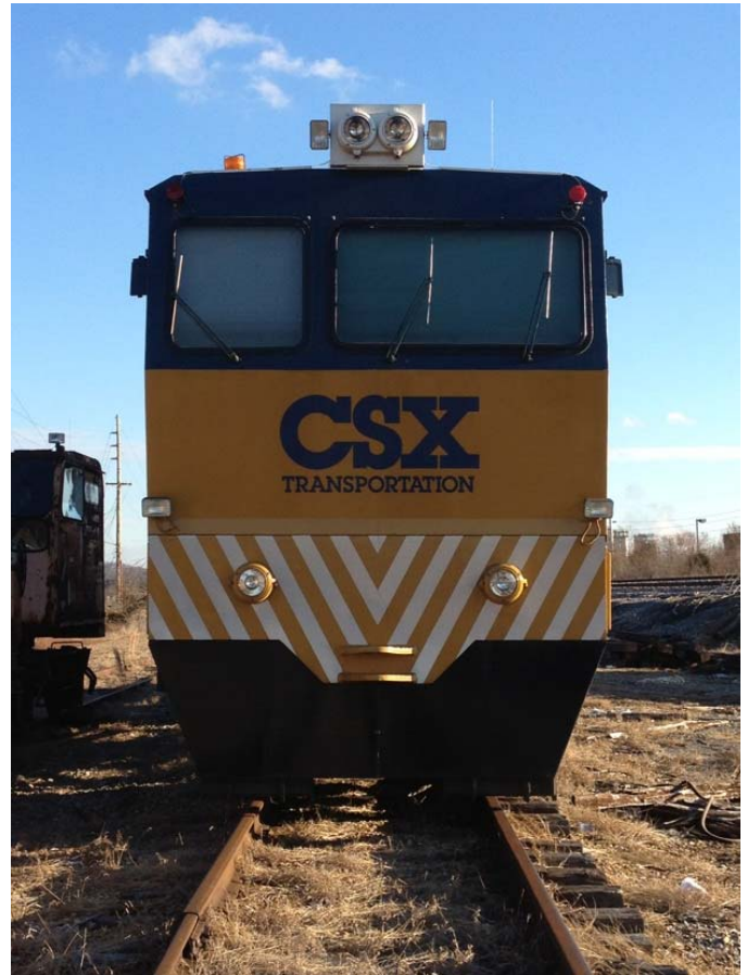
CSX Track Geometry Car
