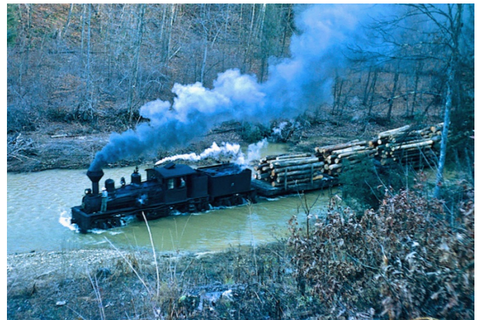
How would you model this – only a steam locomotive could do this. A diesel can short out its traction motors in just 4 inches of water!
