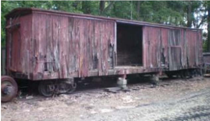
East Tennessee & Western NC #434- This rare car ran between Johnson City, TN and Boone, NC along the famous "Tweetsie" line from 1910 to 1940. At 37 feet long, it is a member of the largest class of narrow gauge boxcars ever built. Its primary duty was hauling cut wood from the timber-rich Blue Ridge Mountains.
