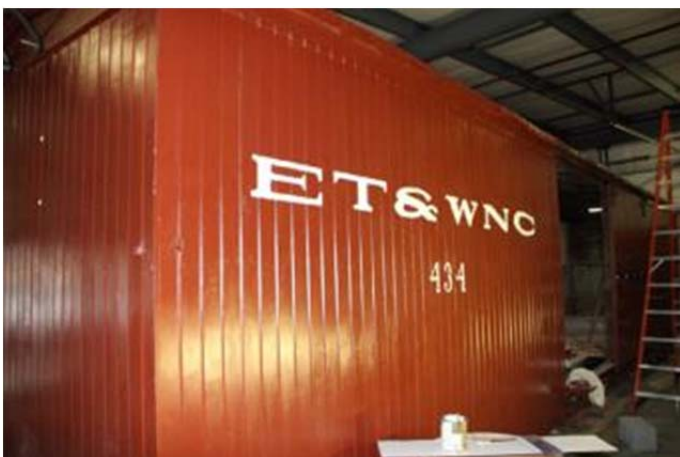
East Tennessee & Western NC #434- This rare car ran between Johnson City, TN and Boone, NC along the famous "Tweetsie" line from 1910 to 1940. At 37 feet long, it is a member of the largest class of narrow gauge boxcars ever built. Its primary duty was hauling cut wood from the timber-rich Blue Ridge Mountains.
