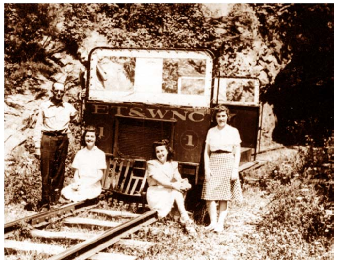
ET&WNC #1- This gang railbus/motorcar was built by the ET&WNC in the late 1920's to haul work crews between Johnson City, TN and Boone, NC. It is being restored to operation and will be a mobile ambassador for the museum.
