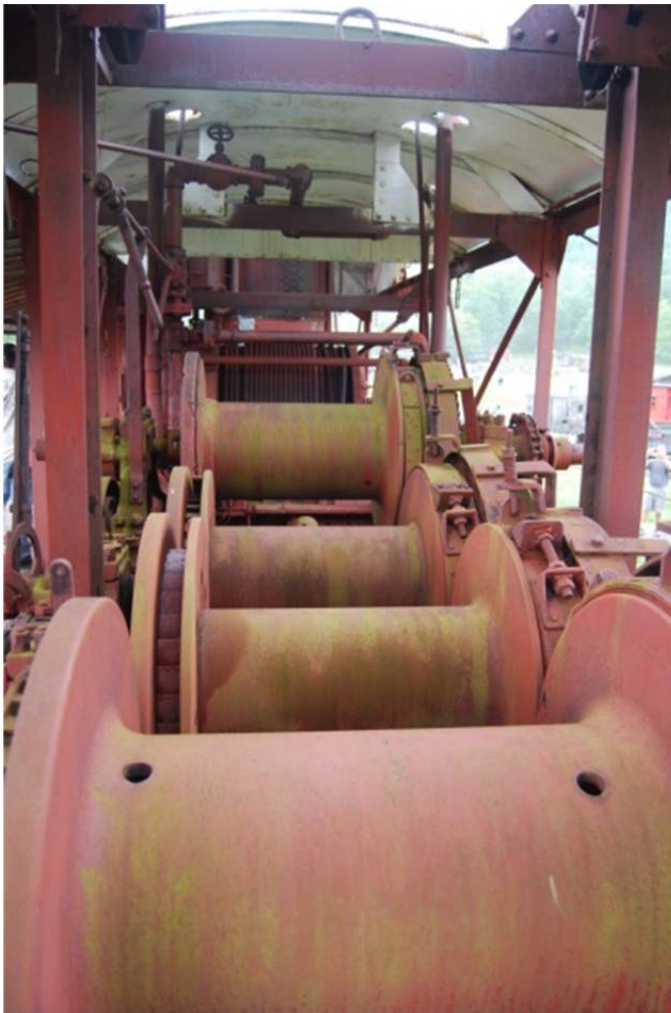
The skidder was built by the Meadow River Lumber Company in 1904 and used until 1966. It was operated by a leverman and a fireman to control the boiler.
