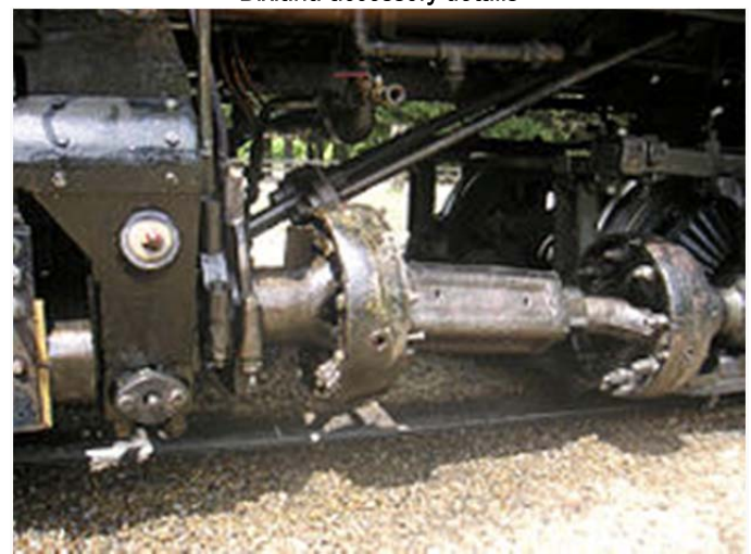
Sonora's universal joints with sliding coupling between
