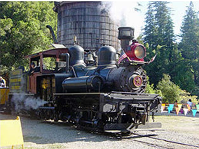
Drive side of the Class B Shay locomotive Dixiana at the Roaring Camp and Big Trees Narrow Gauge Railroad, Felton, California
