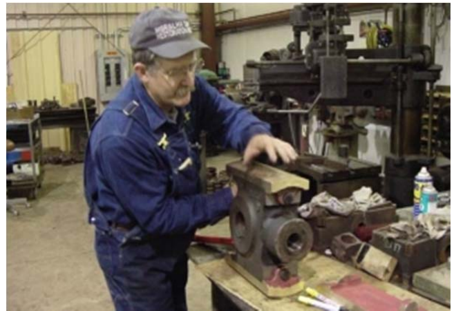
Restoration Project Leader Grady Smith assembling a repaired piston crosshead for the Climax locomotive. (Photo by Gerald Curtis)
