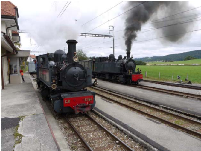
The two locomotives of La Traction ran their earlier lives in north Portugal, on the CP, the state railroad, in the Douro valley; #E206 was built in 1913 by Henschel, works no. 12281, one of 16 in its class, and ran until 1978 in regular service. #E164 was built in 1905, works no. 7022, one of a class of 10, and also ran until
