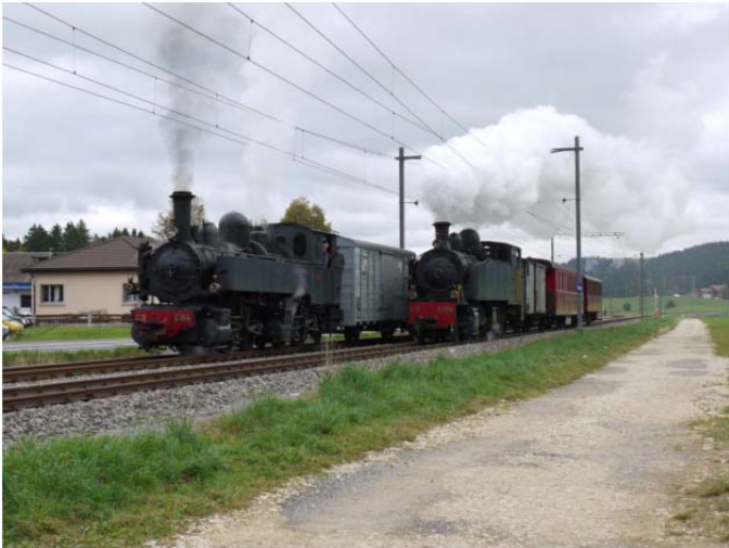
The two locomotives of La Traction ran their earlier lives in north Portugal, on the CP, the state railroad, in the Douro valley; #E206 was built in 1913 by Henschel, works no. 12281, one of 16 in its class, and ran until 1978 in regular service. #E164 was built in 1905, works no. 7022, one of a class of 10, and also ran until
