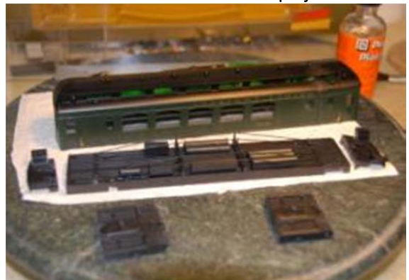
Photo 9: The frame [underbody] is shortened to fit the shell by cutting the step-wells from the ends.
