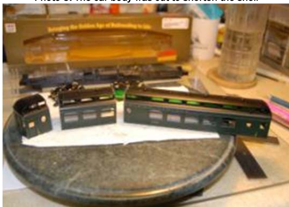
Photo 6: Cut carefully as the center section will be removed
