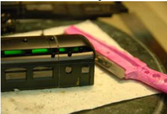
Photo 5: The car body was cut to shorten the shell
