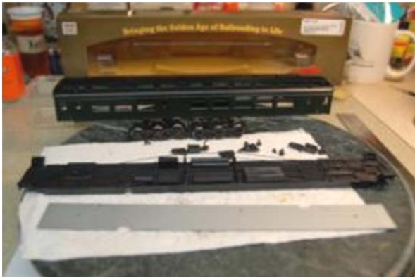
Photo 4: The care was first disassembled removing the under body from the shell and detaching the trucks
