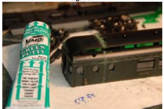
Photo 8: Model putty is used to fill any gaps...Testors and Squadron Green are two sources for tubes of putty.
