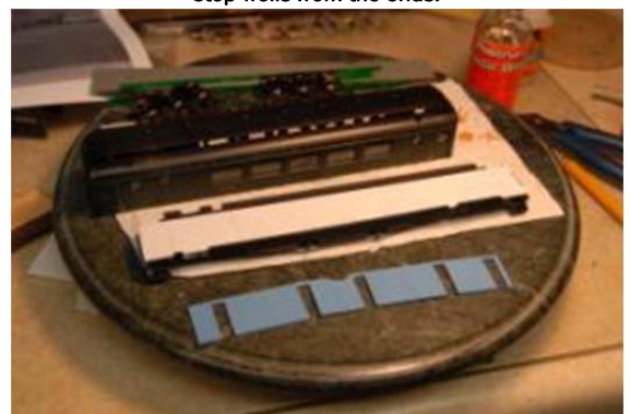
Photo 10: An interior floor is cut to fit and wall panels fabricated to create interior partitions.
