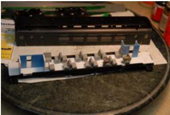
Photo 11: The partitions and seats were fitted and glued to the flooring. Seats came for the scrap bin.
