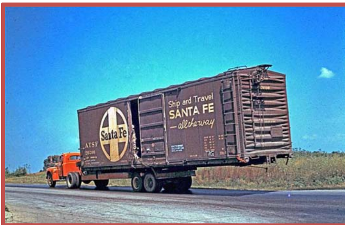
An early try at COT (car on trailer) road service... truck carriers promised to bring car loads to the doors of customers lacking a rail spur. This was a short lived experiment.
