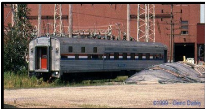
#2052 Dunkirk Harbor (ex-2000, ex-PC 4200, ex-NYC 10810, nee-10364) Budd 16 Dupl. - 1 SR - 10 DBR, rebuilt. from 22 Rmt. (AMTRAK PIX)
