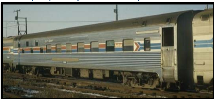
#2004 (ex-2004 Toledo Harbor, ex-PC 4206, ex-NYC 10816, nee-10379) 16 Dupl. - 1 SR - 10 DBR, rblt. from 22 Rmt. (RR PICTURE ARCHIVES)
