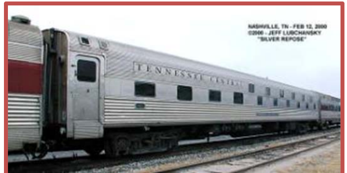
2095 Silver Repose Nashville TN on the Tennessee Central built by Budd 1956 for the Denver Zephyr - ex BN ex CB&Q 4903 ex Amtrak 2023 - renumbered 2095 when converted to head end power - 24 single rooms 8 doubles Photo by Jeff Lubchansky
