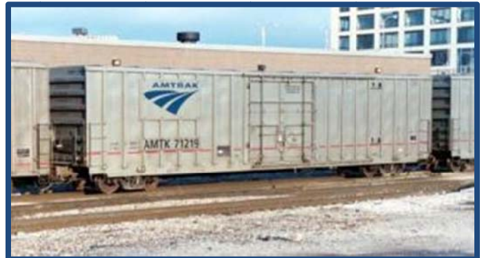
60' Express Boxcars 71200-71299 Built by Trinity Ind. Springfield MO. It looks like they are equipped with electric brakes, delivery started in November 2001.
