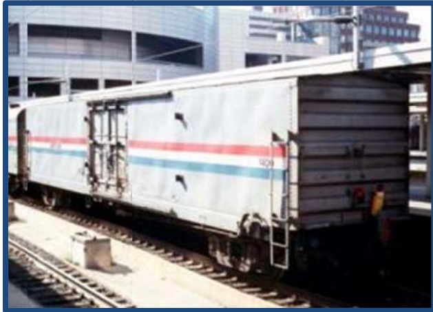
1400-1479 built in 1986 by Thrall - reused old REA Express trucks Mail Handling Cars were embargoed and taken out of service on Feb 11, 2003, and will probably be scrapped.
