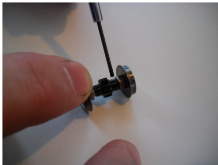
Additional Axle Checks Checking second axle revealed identical problem. Repeat corrective procedure for each axle that is split.
