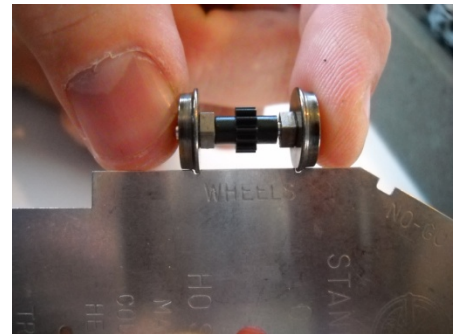
Gauging Wheel-sets Note slight clearance on wheels at gauge
