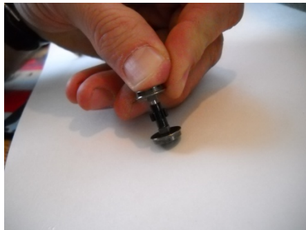
Axle Reassembly Place wheel-sets into each end of gear and press together
