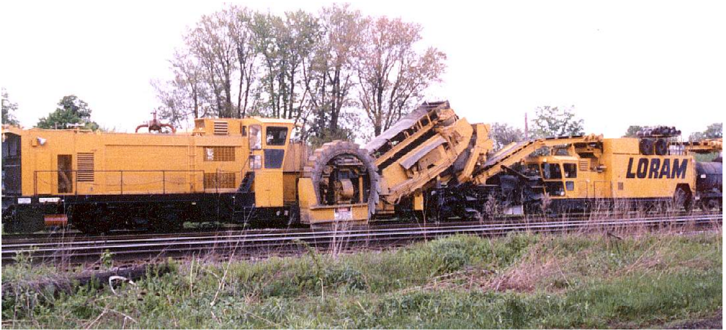
Loram Ballast Cleaner
