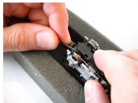
Gear Box Cover removal: Carefully pry up one end of gearbox using precision flat blade screwdriver
