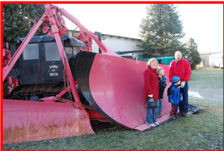
A Best Model 60 (Caterpillar) Highway Snowplow (circa 1924) rests nearby. The tracked snowplow is a 4-cylinder bulldozer with LaPlant-Choate mechanical plow. It was used for many years by the Town of Rush to clear deep snow drifts throughout the town.
